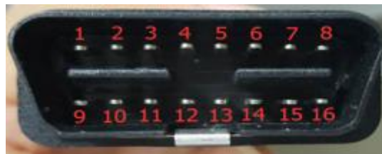
Pic 3: 16 pins on the vehicle OBD connector
